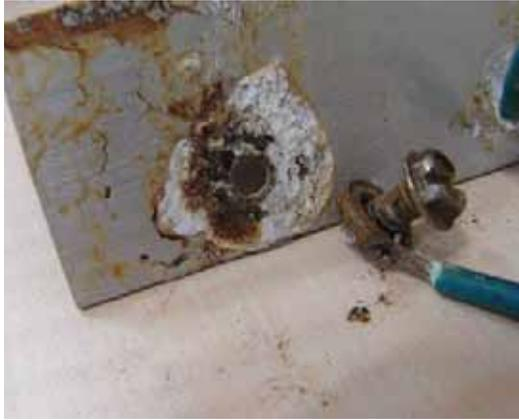
*Figure 9 Build-up of white oxidations on the aluminum frame (screw sample)*
