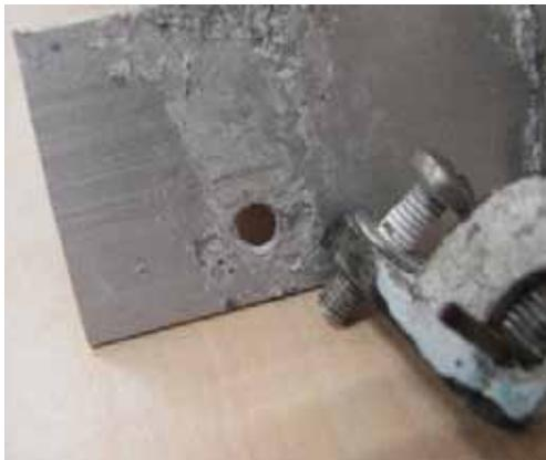
*Figure 10 Build-up of white oxidations on the aluminum frame (lug sample)*
