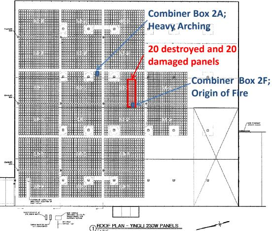
5,252 230-Watt PV modules; Two inverters 500 kW inverters and one 135 kW inverter.
