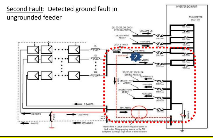
If second fault occurs in an grounded feeder, all current flowing to the inverters (1235 amps) from all of the combiner boxes can be re-routed to the ground and string conductors when GFP trips.
