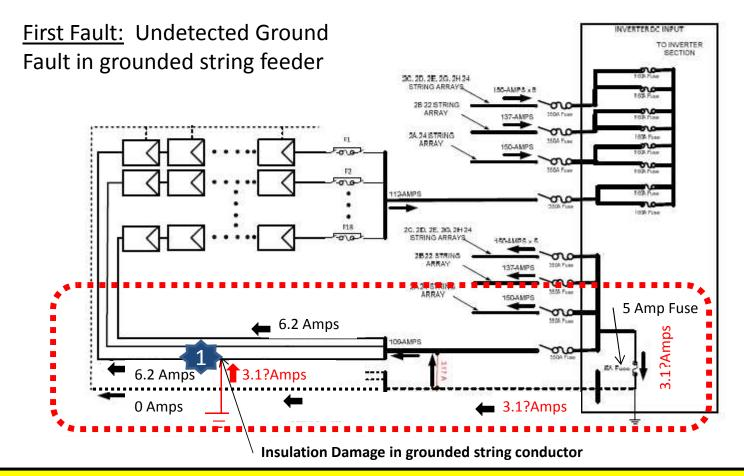
A Ground fault in ungrounded string feeder (normally operating between 6 to 8 amps) can be too low to be detected by the GFP in the inverter when current is split between the feeder and ground (3 to 4 amps).
