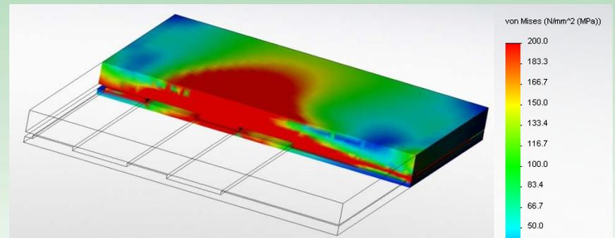
Close up view of glass and busbar junction stress after 2 seconds of arcing on the  $\sim 1/2$  mm<sup>2</sup> connection. Patterned and tempered glass likely shatters at about 100 MPa of tensile stress.
