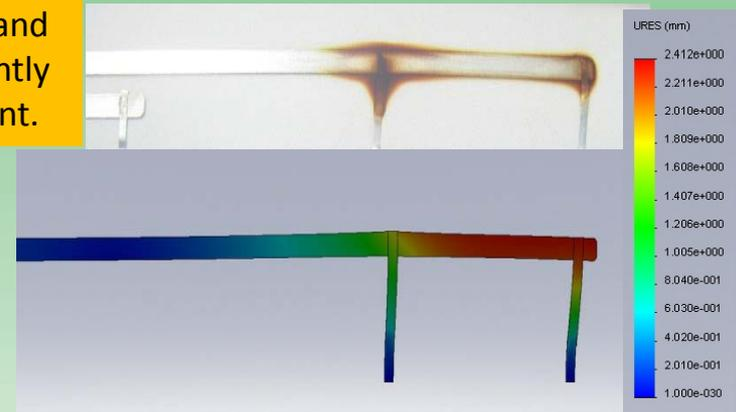
Simulation shows that the region near the arc and to the right is shifted 2 mm after just 1 second of  $\sim\frac{1}{2}$  mm<sup>2</sup> arcing, likely enough to break nearby solder joints
