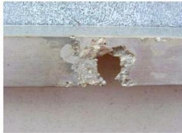
This system is installed on an off-shore island of Taiwan for only 5 years
